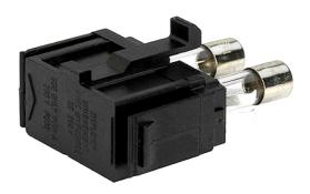
The fuse holder is located on the back of the unit, the fuse must be replaced by a 3.15AT type (5x20mm). Normally the fuse should never blow – if it has, it is a sign of a serious fault condition. Further investigation is needed.
