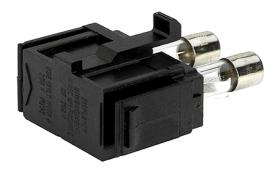
The fuse holder is located on the back of the unit; the fuse must be replaced by a 3.15AT type (5x20mm). Normally the fuse should never blow – if it has, it is a sign of a serious fault condition. Further investigation is needed.
