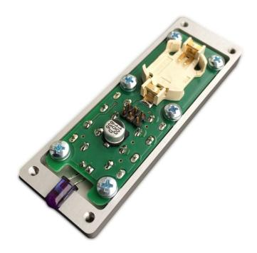
The remote control supplied with the VS 30 is equipped with a CR2032 lithium battery. The battery life is usually more than a year, probably much longer. To replace the battery, the 4x screws on the bottom must be unscrewed. The actual battery is fixed in the holder. (See picture above)
